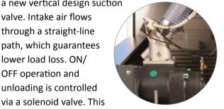
valve concept has been specially designed to keep the number of components down to a minimum, so as to ensure long-lasting durability and low maintenance requirements.
